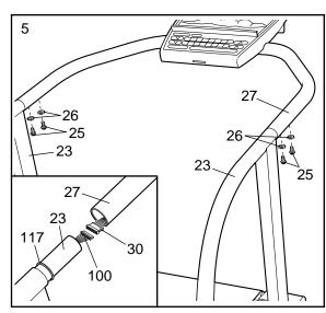
Tighten all of the bolts used in steps 4 and 5.
